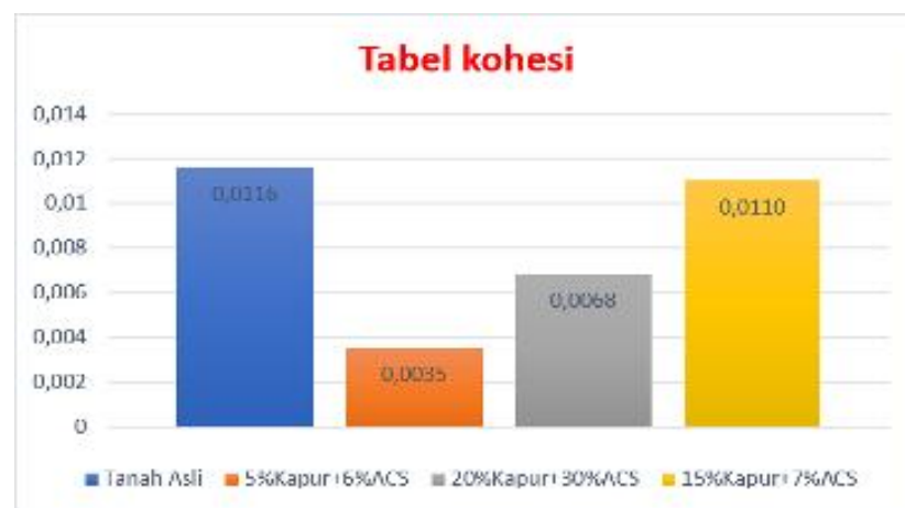
Gambar 4. 7 Diagram batang variasi campuran kohesi
