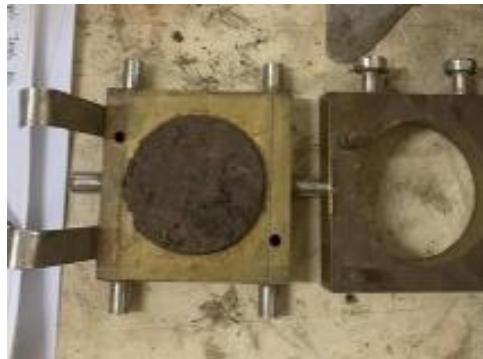
Gambar 3. 29 Persiapan benda Uji direct shear
