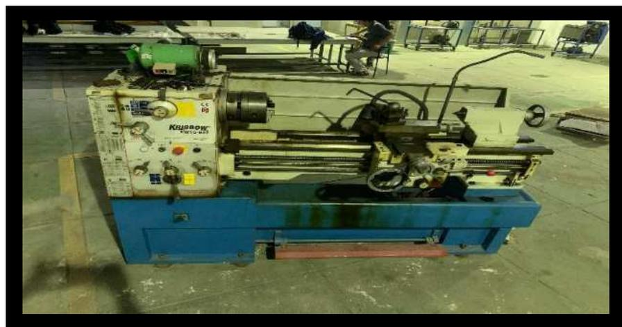
Gambar 3.2 Mesin Bubut type Krisbow KW15-907.
