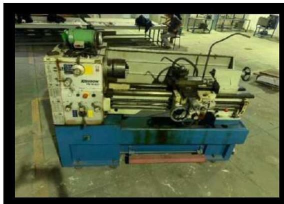
Gambar 2.3 Mesin bubut Krisbow KW15-907
