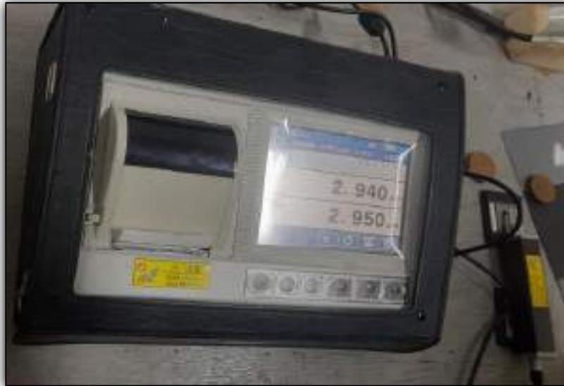
Gambar 3. 6 *Surface Raoughness tester*
